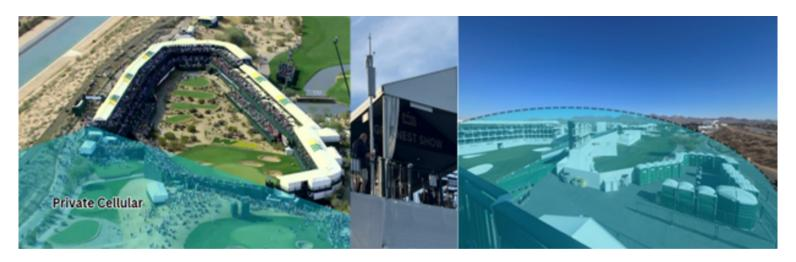
The team used three routers to provide Wi-Fi 6 (5Ghz/2.4Ghz) coverage across all three floors of the WM suite portion of hole 16. Each router was strategically placed on a different floor, ensuring seamless connectivity and load balancing for event staff, VIP guests, and operational devices.
